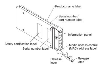
For more information about the components of the information panel, see Chapter 3, "Information panel LEDs and external Fibre Channel ports," on page 27. For more information about the MAC address, see the applicable QuickTools switch management guide on the *QLogic 8 Gb Intelligent Pass-thru and SAN Switch Modules for IBM BladeCenter Support* CD or at http://support.qlogic.com.
